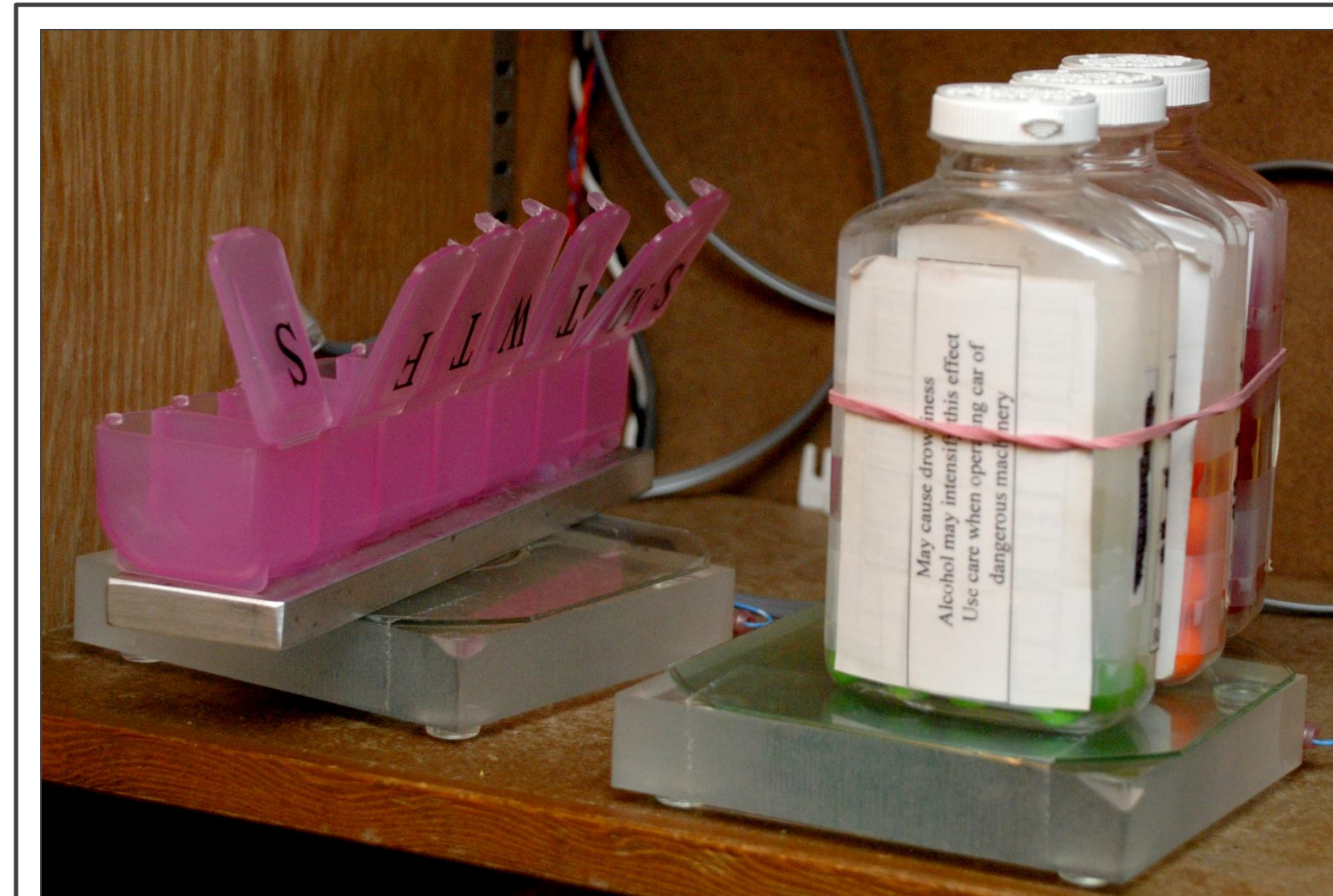
Object interaction sensors inside a kitchen cabinet. Senses the presence or absence of an item, based on small discrepancies in weight.
