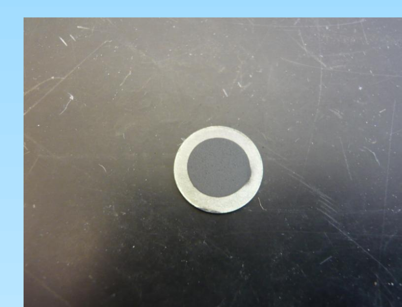
Sintered Fuel Cell With Cathode and Silver Paint
