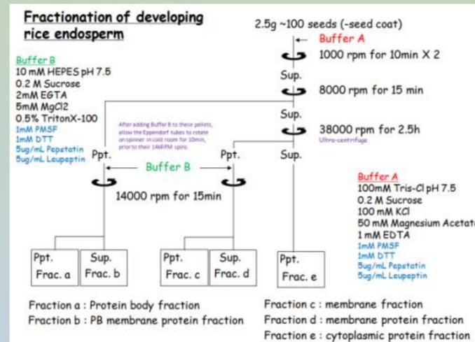
**Figure 2.** Schematic representation of the fractionation protocol performed on developing rice endosperms. The cytosolic fraction E of both wild type and gluP6 was protein assayed to quantify yield and concentration of protein.
