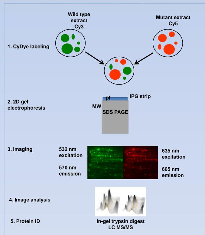
**Figure 3.** The diagram shows a schematic representation of the 2D DIGE analysis performed on wild type and *gluP6* mutant developing rice seed extracts using CyDye fluors (GE Healthcare). Differentially expressed protein spots were excised, in-gel trypsin digested, and analyzed by liquid chromatography tandem mass spectrometry.
