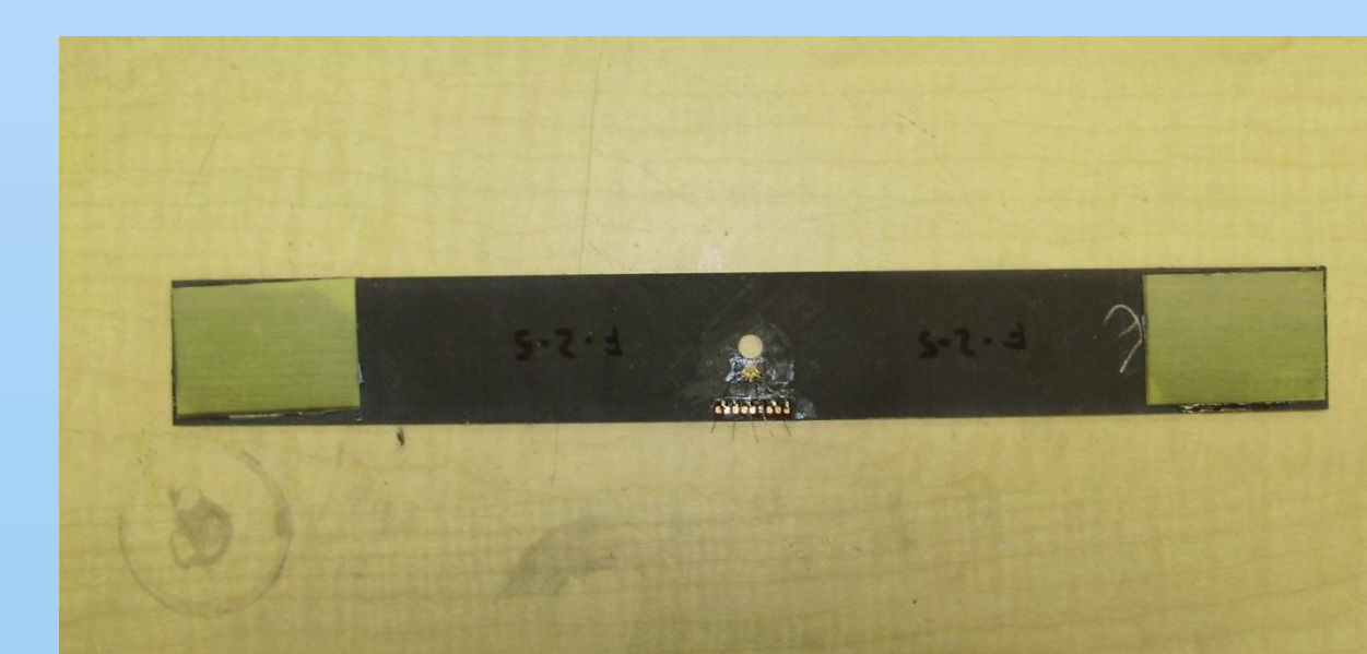
A coupon with strain gage attached
