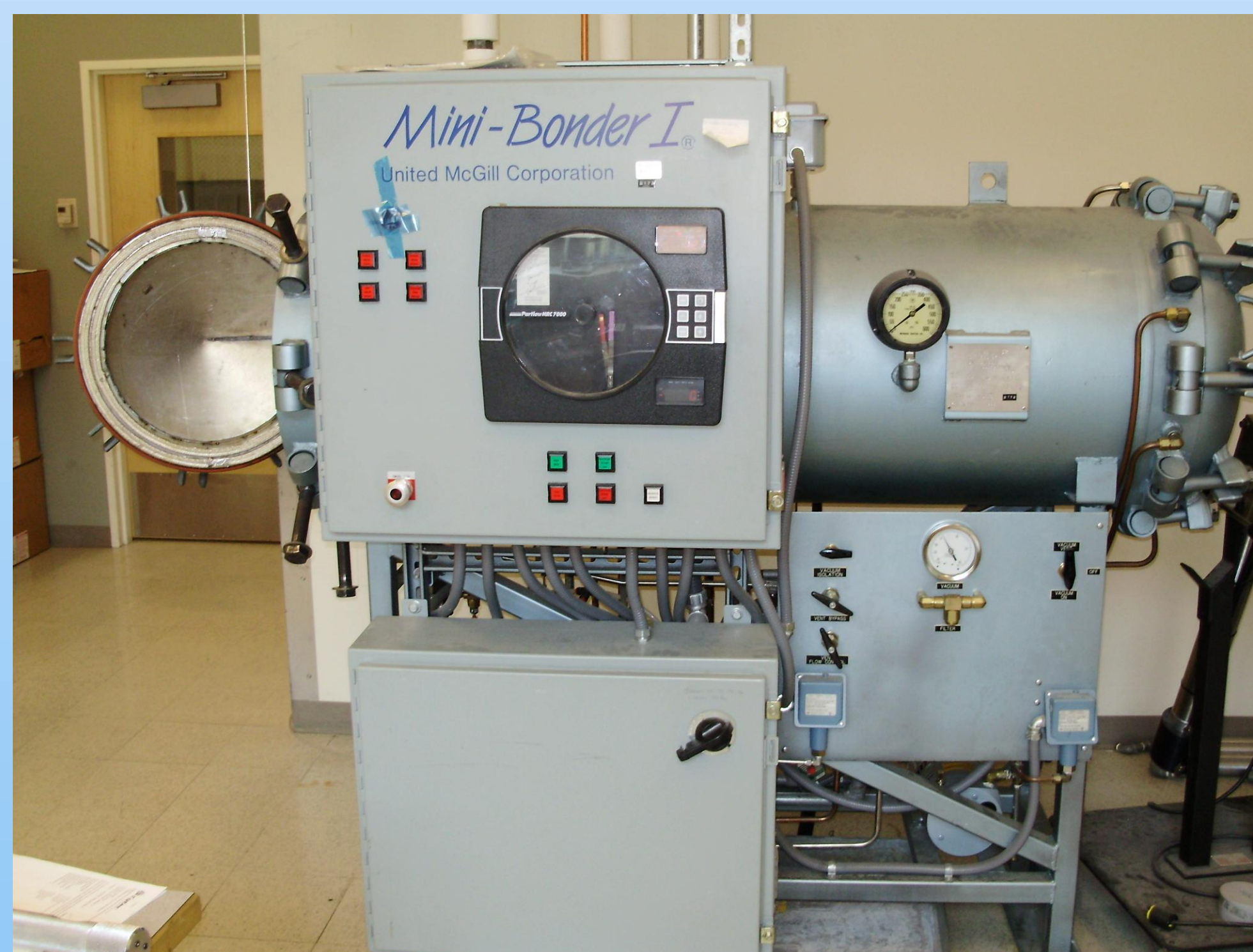
The Autoclave used to cure the composite plates
