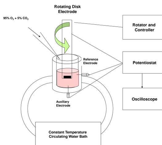
**Figure 4.** The setup of the rotating disk electrode with tissue in chamber.
