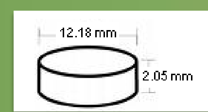
500 mg powder pressed at 145 MPa for 1 minute
