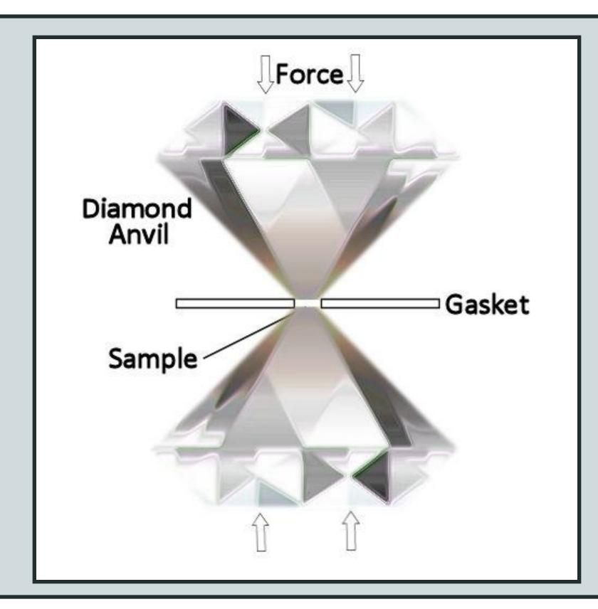
Ruby fluorescence is the most common technique used to measure pressures with more accuracy. When a ruby is placed under pressure, a peak in its red fluorescence spectrum shifts to a higher wavelength. The peak location is measured for a reference ruby at atmospheric pressure and for a ruby chip included in the cell, and the difference in wavelength is used to calculate the pressure within the cell.
