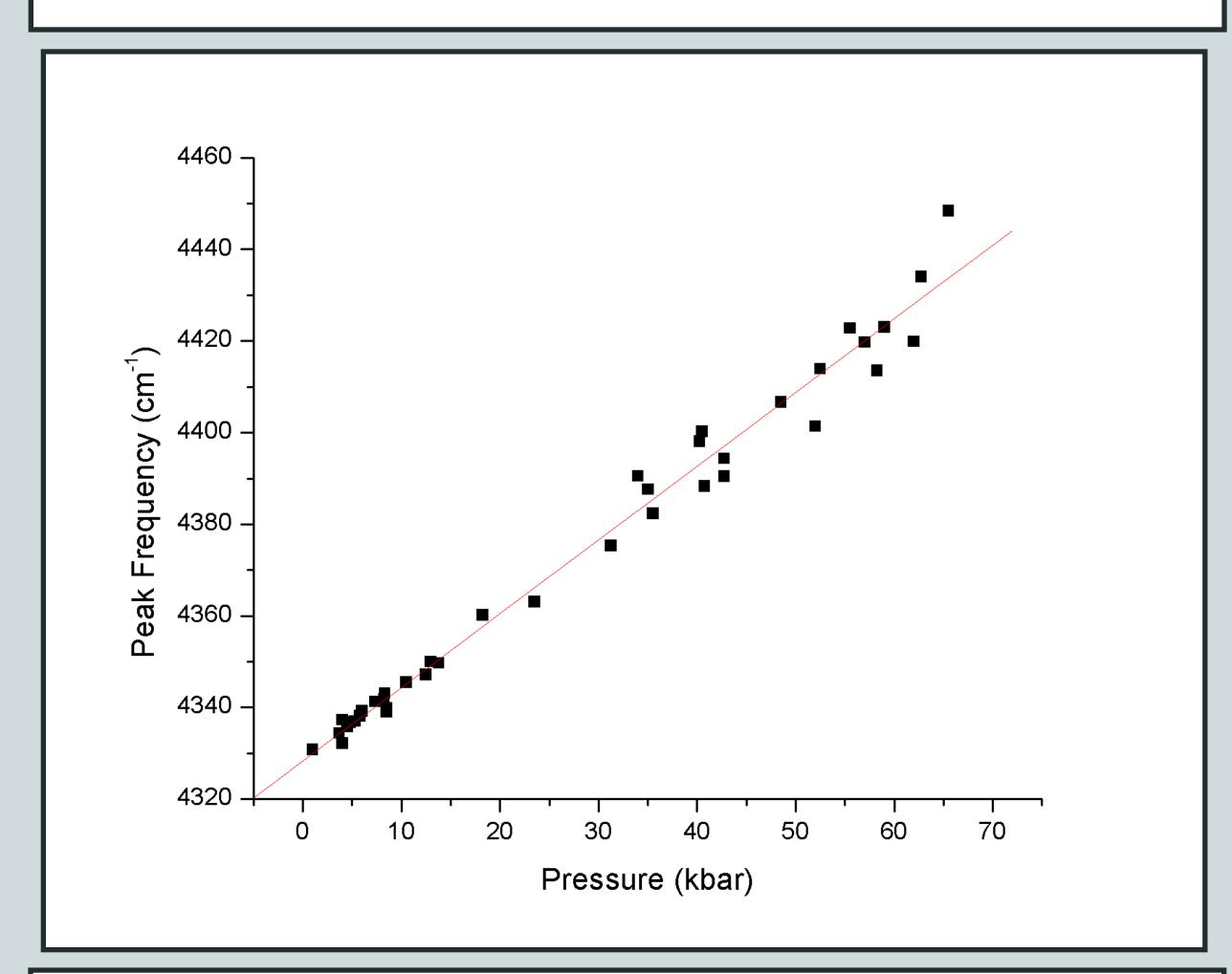
The position of this peak in the infrared absorption spectrum of mineral oil appears to be a reasonably accurate indicator of the pressure in the cell. More data are needed to improve the equation and the accuracy of calculations. By observing the location of the peak in many more spectra to better establish the linear relationship, it should be possible to determine the pressure on diamond anvil cell samples that contain mineral oil, without the need to include a ruby chip.
