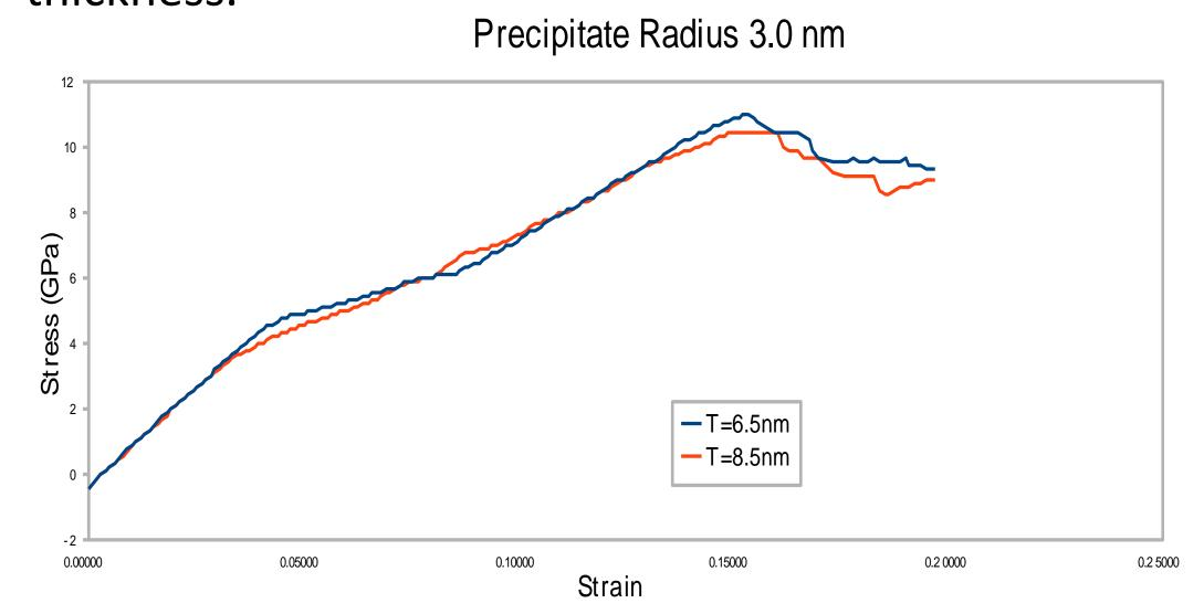
• By changing the size of the precipitate, a thicker material can be made as strong as a thinner material. Adding precipitates to Cu-Nb multilayer composites will help to improve the performance of these materials.
