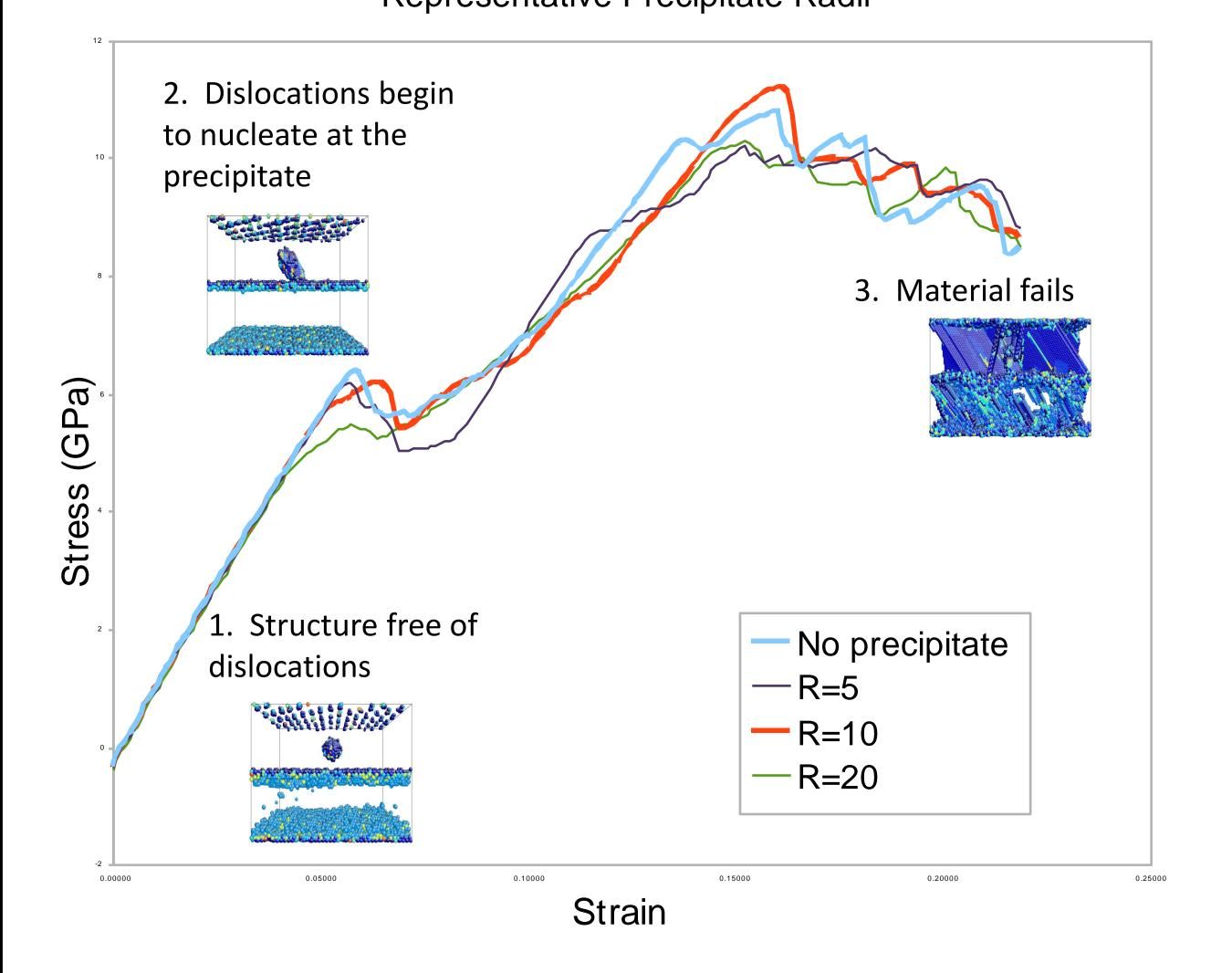
• The stress-strain curves indicate that the size of the precipitate determines whether the material strengthens or weakens
